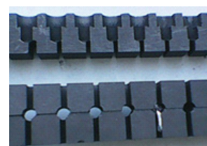
Fig. 7. Photograph of the upper and lower parts of the graphite cassette used to form “ n -Si — Al+Si melt — p^+-Si ” structures
